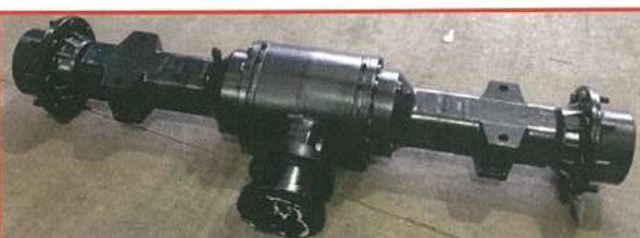
Single hydrostatic drive motor coupled to a JCB differential axle ensures reliable continuous drive for long distance travel
